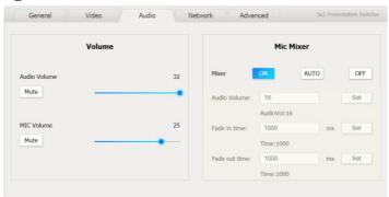
This page is for controlling the audio volume levels and the microphone mixer section. The values in the lower portion of the **Mic Mixer** block can only be changed when the **AUTO** mode is active. The Mic Mixer portion controls the automatic behaviour of the in-built audio ducking function
