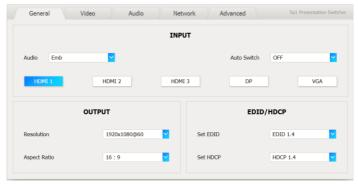
This page provides basic control of the video switcher and audio input selections. Control for output resolution, input aspect ratio, auto switching mode, EDID and HDCP settings are also provided.
