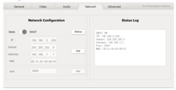
The network page provides information for the current IP settings. Note that the values in the Network Configuration section can only be changed when the IP mode is set the **Static**. To change the mode, click the sliding button to the preferred setting. Use the **Status** button to refresh to the current settings.
