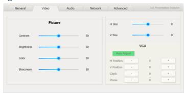
This page allows for adjustment of the output video to the HDMI OUT and HDBT OUT ports. It also permits control over adjustments for the VGA input.
