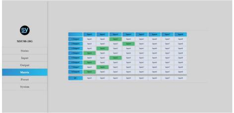
This image shows the factory default names. The number to the left of the output names is always automatically added to indicate the actual output number.
