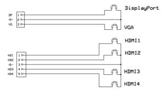
For each connector, pin 1 is left-most when viewed from the rear of the MFT62.
