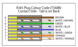
Ensure that the cable terminations are correctly wired and properly crimped before inserting the cable connector into the HDBT output port of the MFT-62.
