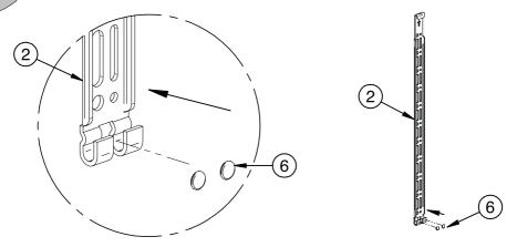
Attach the interface arms to the back of the flat screen.
